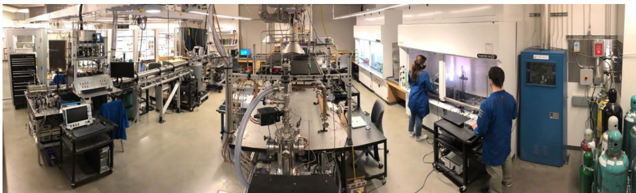
A picture of the Spearrin lab at UCLA c. 2024. On the left we see the long metallic shock tube that can create combustion environments (high pressure and high temperature explosions recreated inside the tube chamber). The shock tube is an essential tool for scientists who want to carry out combustion diagnostics in the lab.
