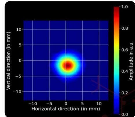
Left: Picture of the fiber-coupled HHL-packaged QCL. Right: Beam profile right after the fiber exit.
