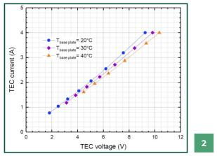
Current-voltage characteristics of the built-in TEC for different temperatures of the base plate.
