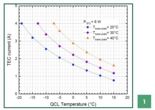
TEC current consumption as a function of the wanted QCL chip temperature for different base plate temperatures and for a QCL thermal load of 6 W.
