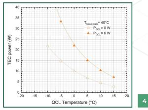
Power consumption of the built-in  $TEC^1$  as a function of the QCL chip temperature for a base plate temperature of +40°C, with and without a thermal load in the QCL.
